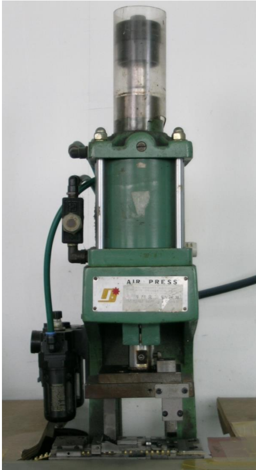
Terminal Caulking M/C
